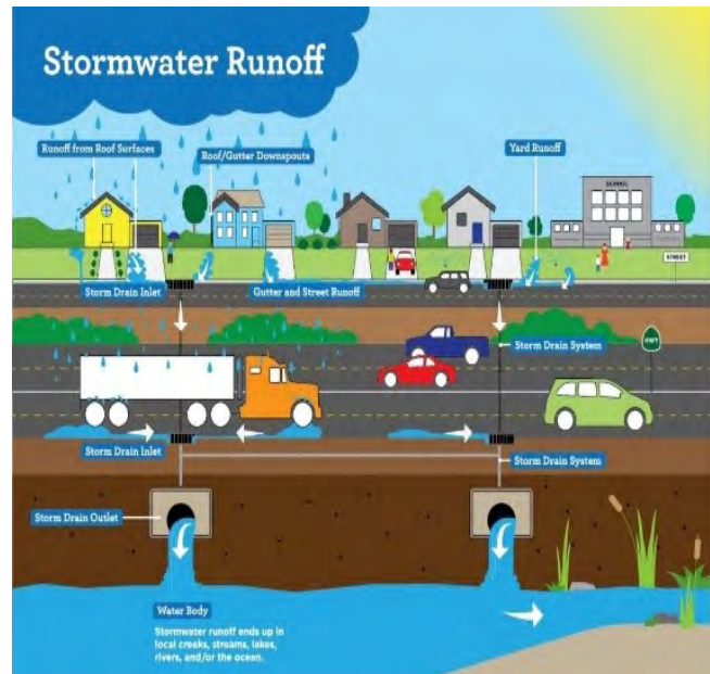
Illustration of stormwater runoff
